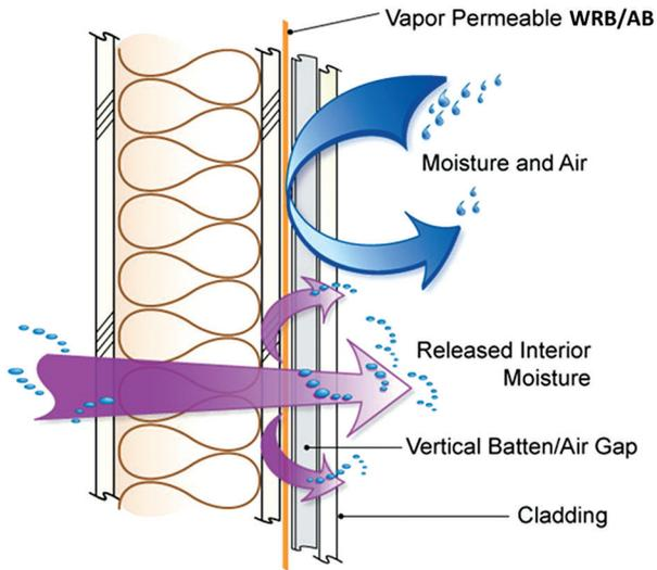
**Figure 8 – Vapor-permeable WRB/AB membrane, allowing wetted interior materials to dry to the exterior via vapor diffusion. In addition, both sides of the cladding can dry, reducing any moisture loads.**
