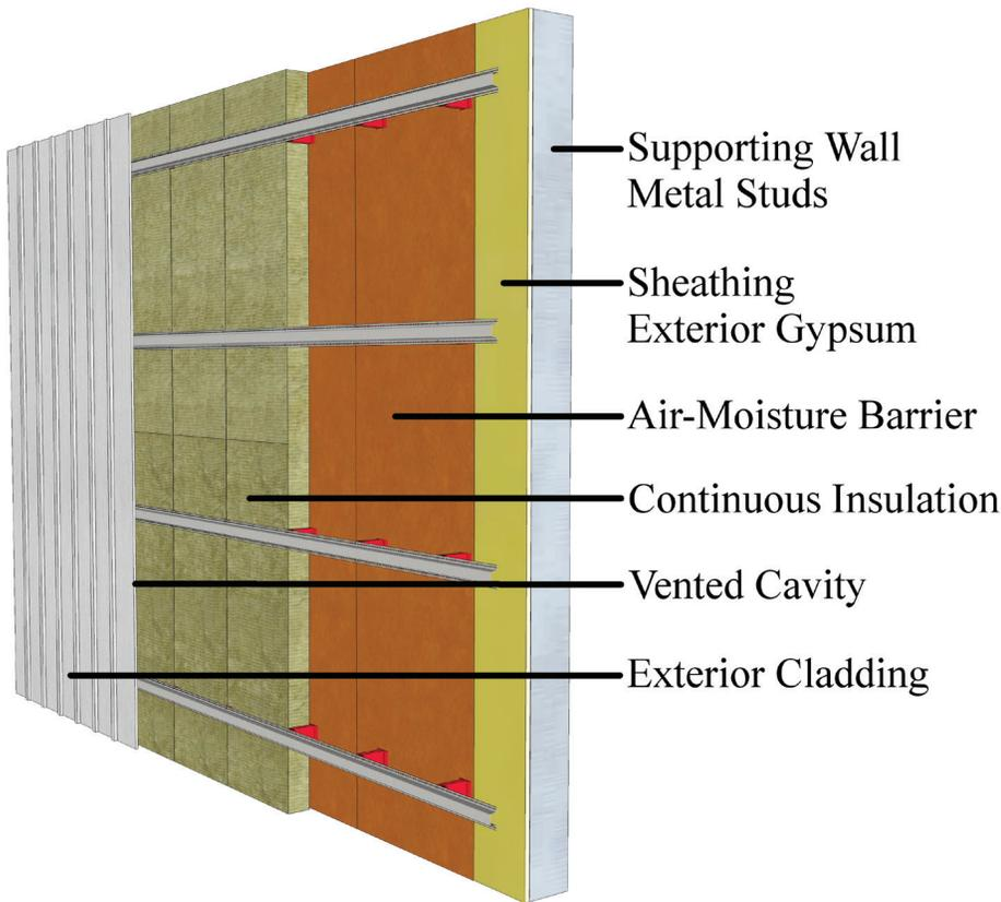
**Figure 3 – Common commercial wall assembly overview of a rainscreen system.**
