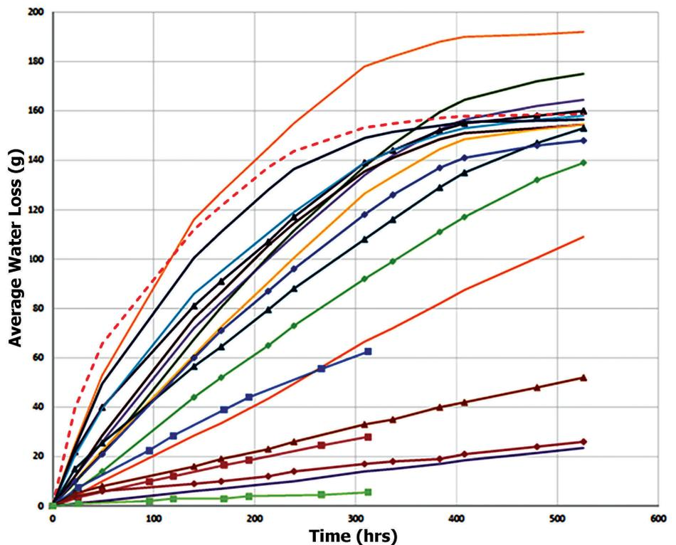
**Figure 10 – Plot of sample weight versus time (0-600 hours), demonstrating moisture loss of drying plywood wrapped or coated with common fluid-applied and membrane WRBs.**
