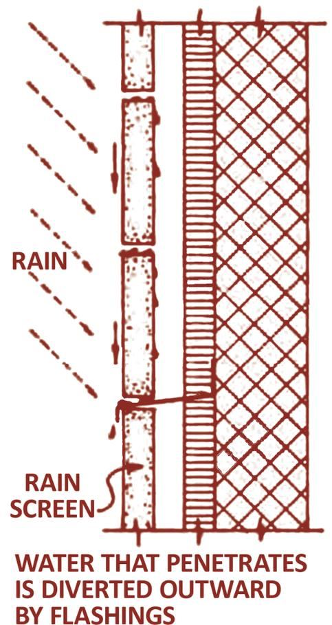
*Figure 2 – Hutcheons' details of a rainscreen system and a typical wall overview.<sup>24</sup>*
