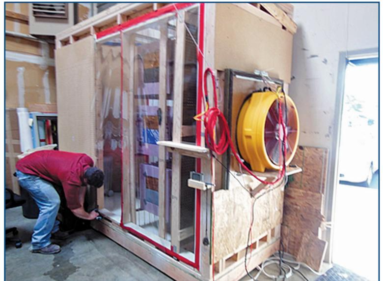
**Figure 9 – Image of the test chamber used in drying studies of plywood samples wrapped in WRB material. Air exchange rate of 50 ACH was used, as it represents the likely flows associated with a properly vented 1/2-in. rainscreen cavity, based on previous research by others accounting for thermal-induced convection buoyancy and typical wind-driven air pressures.<sup>24,25</sup>**
