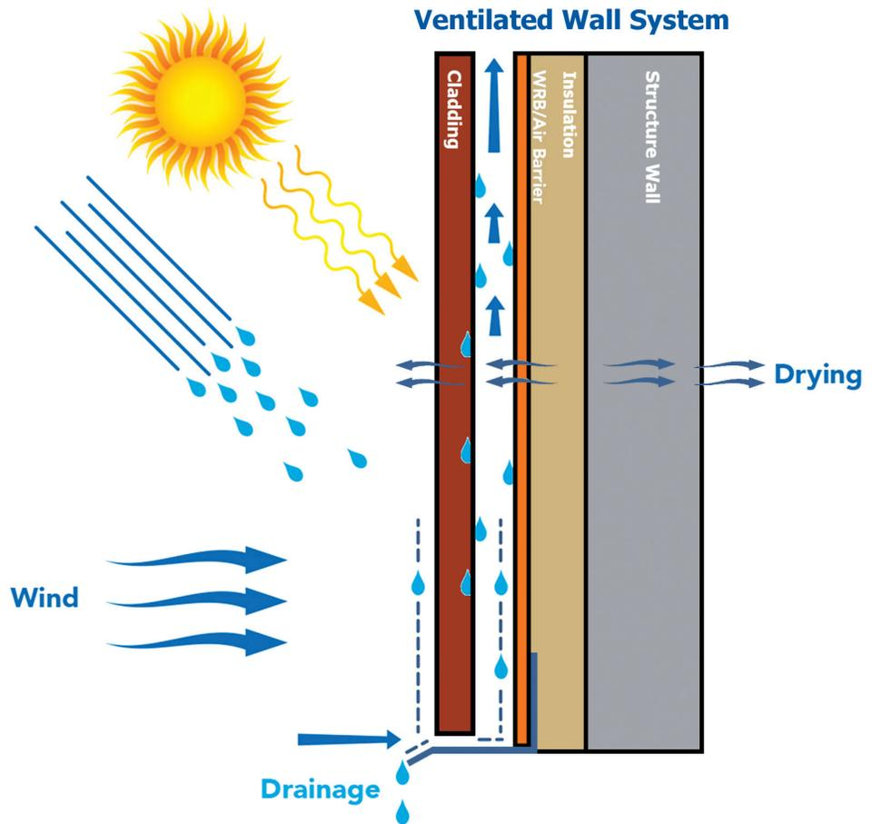
Figure 5 – Vented rainscreen system, providing additional drying by vapor diffusion and venting.
