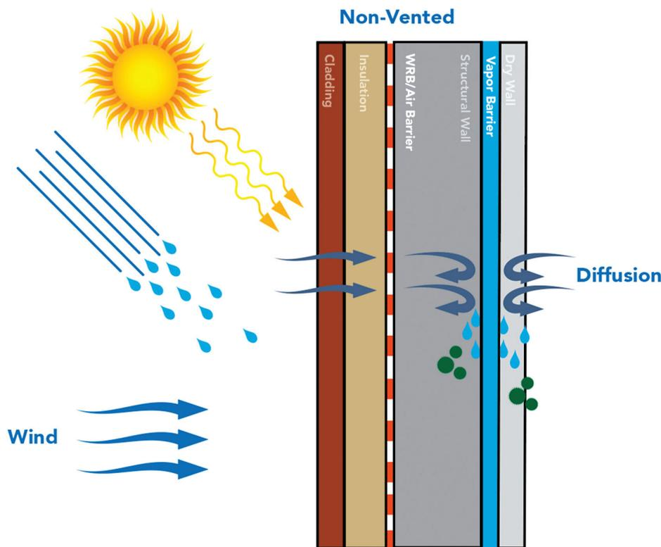
Figure 7 – A non-vented wall system with internal vapor barrier showing condensation due to lack of vapor diffusion at the vapor barrier.
